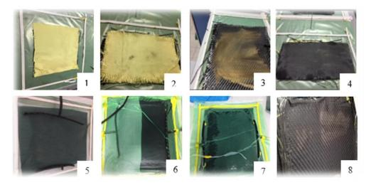
**Figure 4**. (1) spreading of mold release film, (2) laying of fibers,(3) spreading of shell powders, (4) completion of laying process, (5) fixing the elements of the mold, (6), Impregnation of the mixture, (7) curing process, (8) procuded sample
