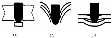
**Figure 1**. The types of ballistic impact (1) Delanimation (2) Fiber breakage (3) Matrix breakage [13]
