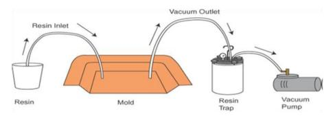
**Figure 2.** The vacuum infusion process main elements [20]
