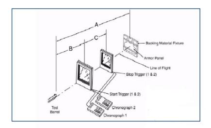
Figure 5. Ballistic experiment setup
