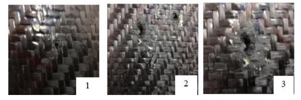
**Figure 9**. Ballistics test result of GNFKC sample (1) Shots 1 and 2,
