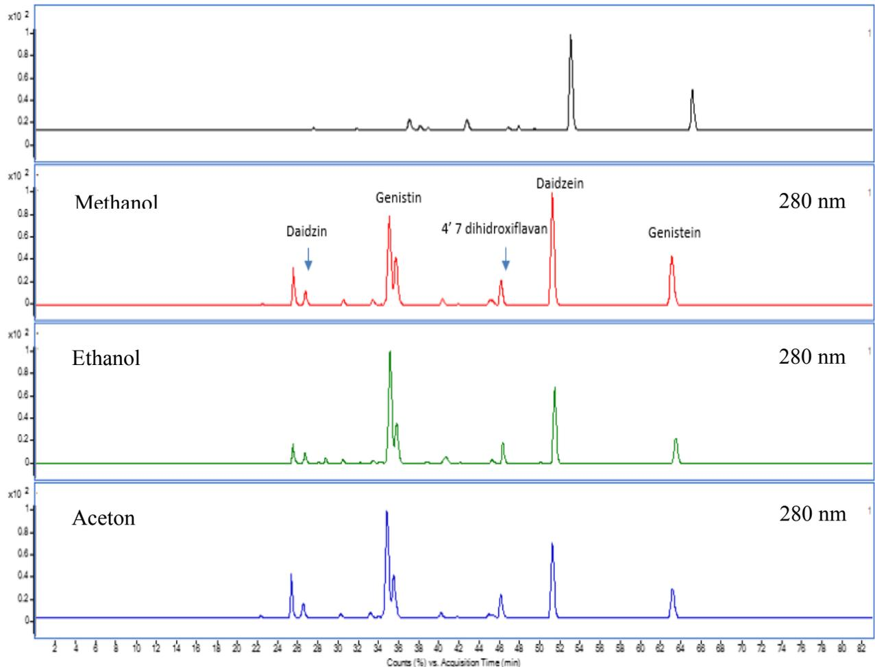
**Figure 1.** HPLC chromatogram of soybean extracts obtained using different solvents
