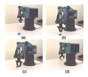
Fig. 13. Action of robot arm for grabbing objects.
