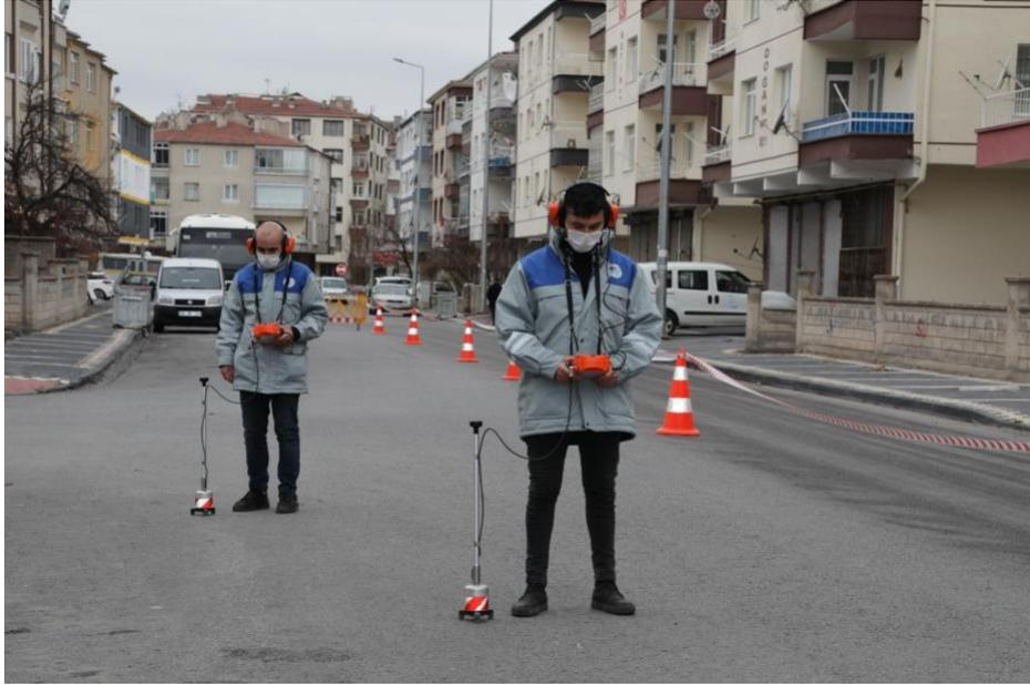
Figure 2: Sample Fault Detection Process with ground microphone
