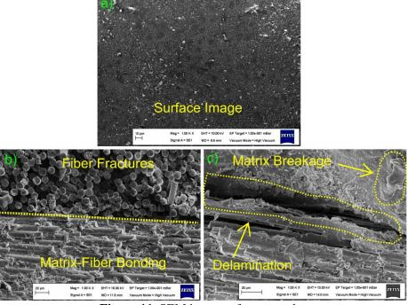
Figure 11. SEM images of test sample
