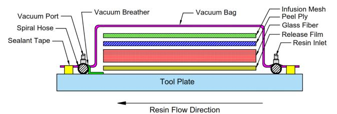
Figure 1. Schematic representation of VARTM
