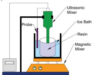
Figure 3. Schematic representation of UMM method
