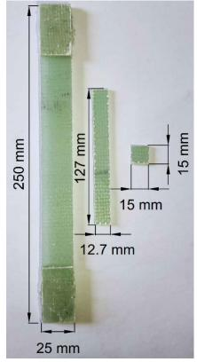
Figure 4. Test samples and dimensions
