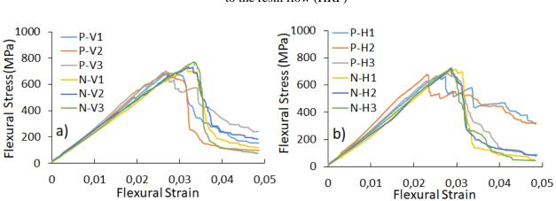
**Figure 9.** Flexural strength-strain curves of composite plates a) vertical to the resin flow (VRF) b) horizontal to the resin flow (HRF)
