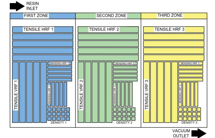
Figure 6. Sampling orientation of composite
