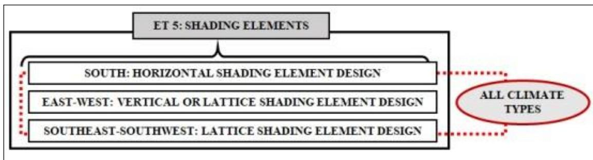
Figure 10. Design guide evaluation topics 5 (ET5), Shading elements
