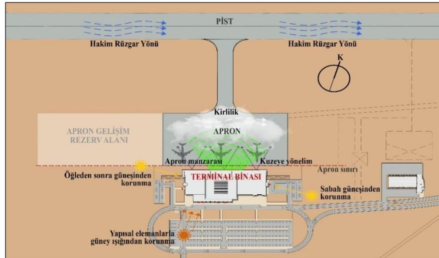
**Figure 15.** Terminal building layout according to bioclimatic data
