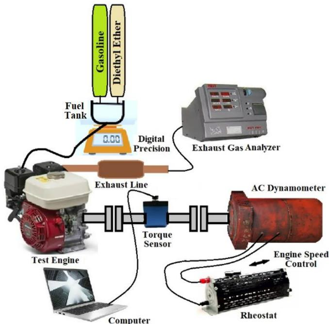
Fig. 1. Schematic view of the engine test setup
