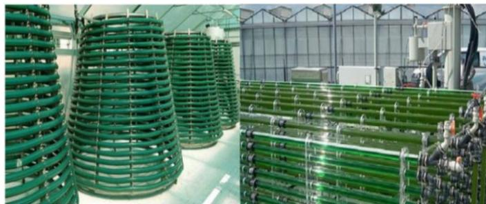
**Figure 5.** Horizontal (flat) production system in photobioreactor (Gezici, 2012).
