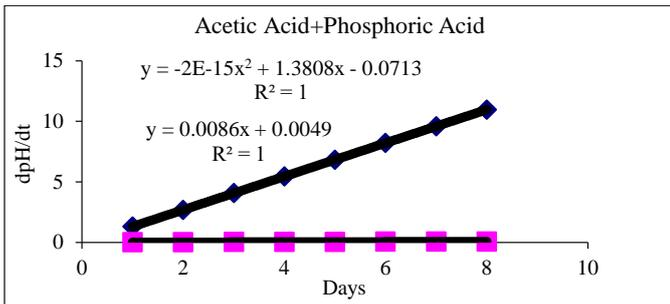
**Figure 27.**  $\frac{dpH}{dt}$  vs  $t$  changes for acetic acid + phosphoric acid mixture
