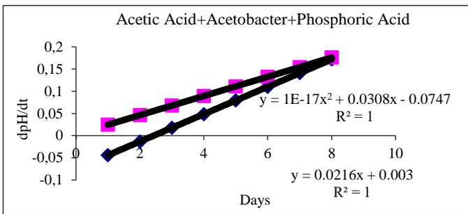
**Figure 19.**  $\frac{dpH}{dt}$  vs  $t$  changes for acetic acid + *A. aceti* + phosphoric acid mixture
