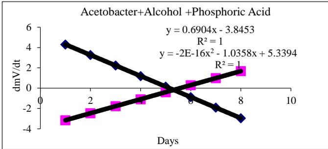
**Figure 26.**  $\frac{dmV}{dt}$  vs  $t$  changes for *A. aceti* + alcohol + phosphoric acid mixture
