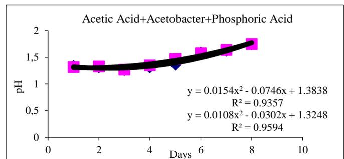
Figure 3. pH changes for acetic acid + *A. aceti* + phosphoric acid mixture
