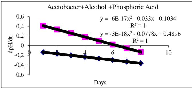
**Figure 25.**  $\frac{dpH}{dt}$  vs  $t$  changes for *A. aceti* + alcohol + phosphoric acid mixture
