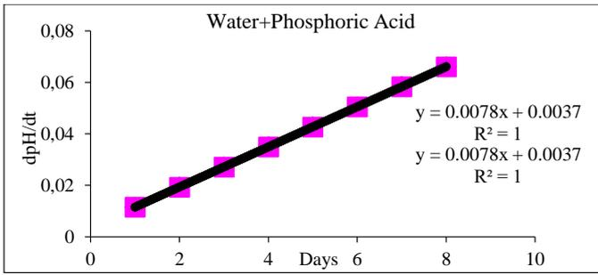
**Figure 17.**  $\frac{dpH}{dt}$  vs  $t$  changes for water + phosphoric acid mixture
