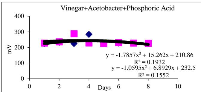
**Figure 6.** mV changes for vinegar + *A. aceti* + phosphoric acid mixture
