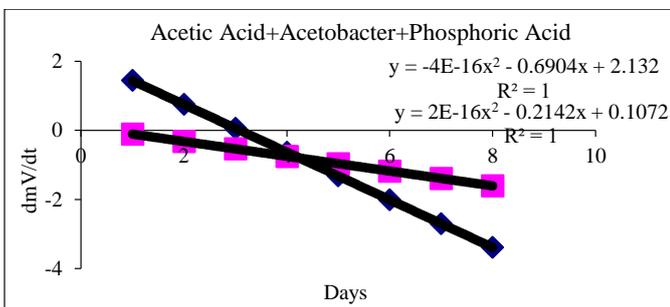
**Figure 20.**  $\frac{dmV}{dt}$  vs  $t$  changes for acetic acid + *A. aceti* + phosphoric acid mixture
