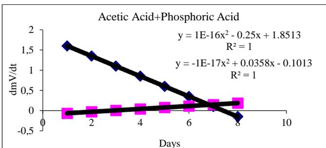
**Figure 28.**  $\frac{dmV}{dt}$  vs  $t$  changes for acetic acid + phosphoric acid mixture
