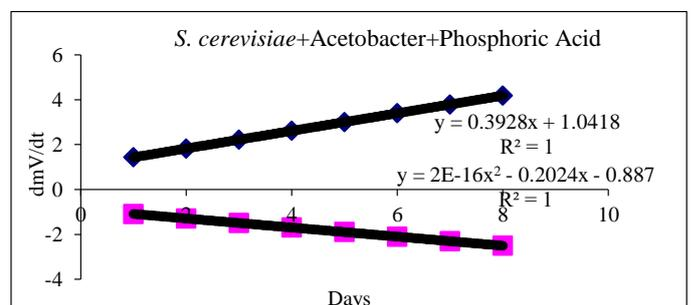
**Figure 32.**  $\frac{dmV}{dt}$  vs  $t$  changes for *S. cerevisiae* + *A. aceti* + phosphoric acid mixture
