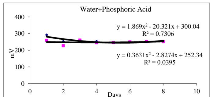
Figure 2. mV changes for water + phosphoric acid mixture
