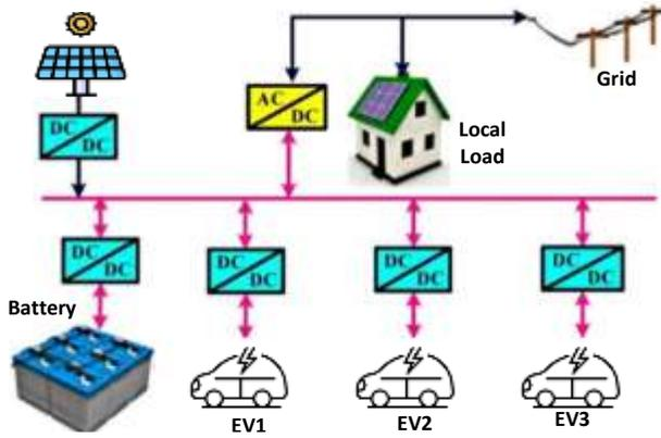
Fig. 4 Representative V2G and V2H systems in different countries [49,50]. The challenges and opportunities in the future development of V2G and V2H technologies for EVs are summarized in Table 4.
