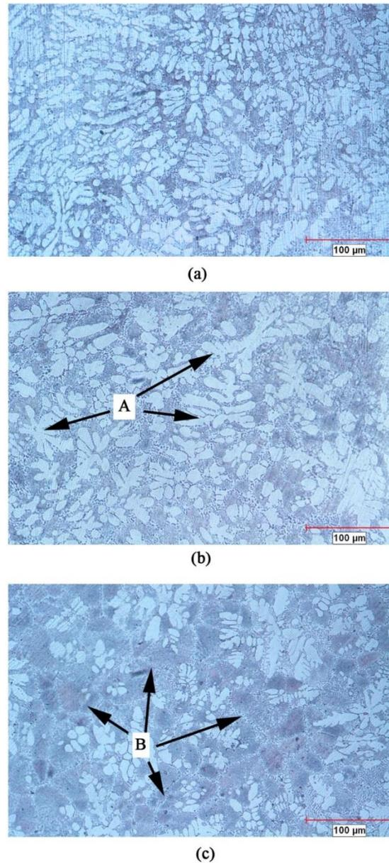
**Figure 1.** Microstructure images of the samples (Optical Microscope, magn. 200X), (a) Base alloy, (b) Z5-0.01Ti (Alloyed at 450 °C and re-melted and cast at 650 °C), (c) Z5-0.03Ti (Alloyed at 650 °C and re-melted and cast at 650 °C).
