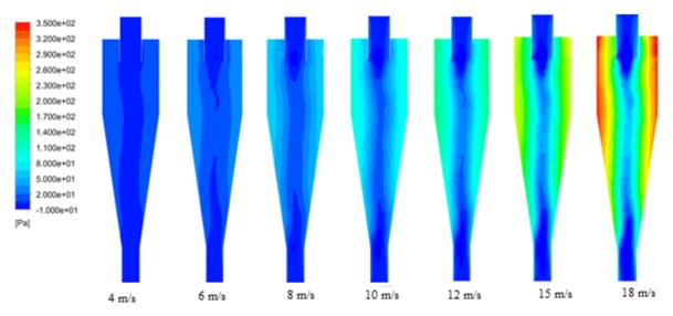
Figure. 4. Pressure distributions in the cyclone of different inlet velocities.
