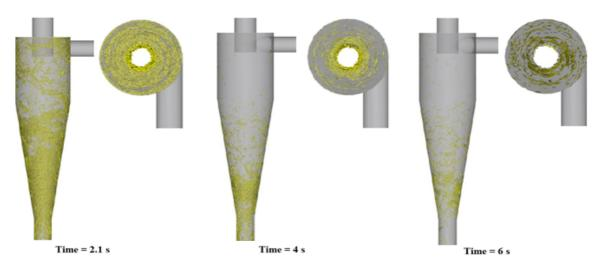
Figure 6. Time-dependent movement of straw in the cyclone at an inlet velocity of 10 m/s.
