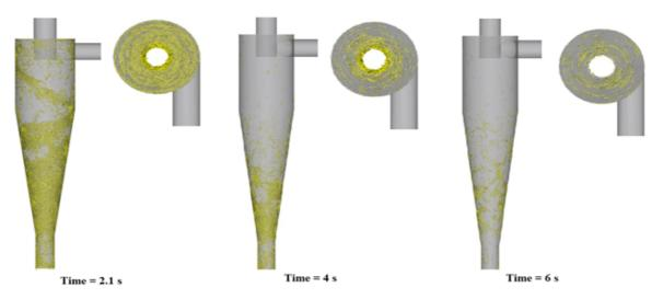
Figure 5. Time-dependent movement of straw in the cyclone at an inlet velocity of 4 m/s.
