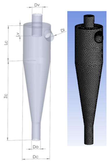
Figure 2. Cyclone model and mesh network.
