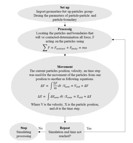
Figure 1. Flowchart of the discrete element method.
