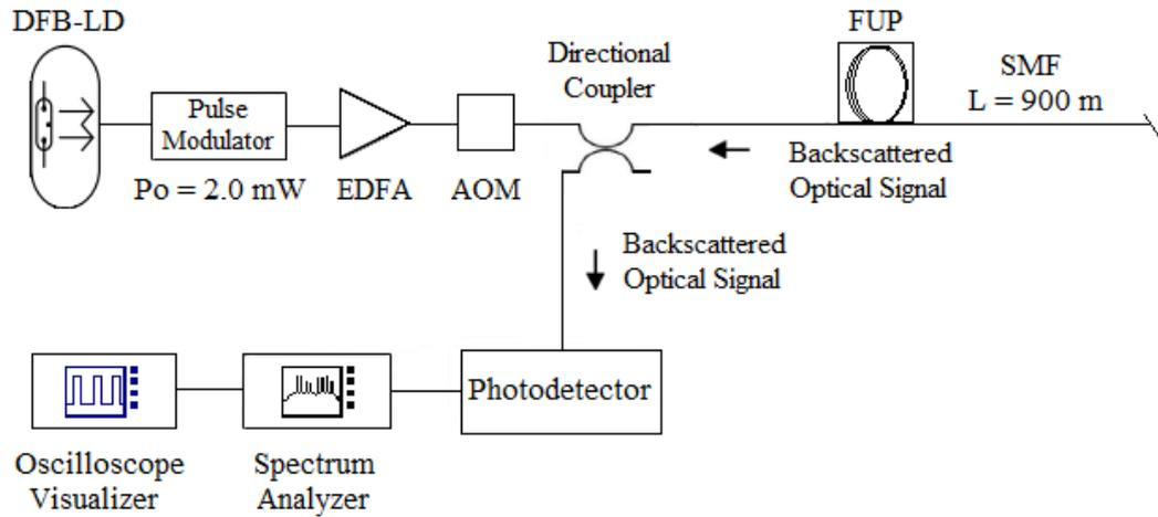
Figure 1. Optical fiber-based distributed pressure sensing (DPS) model
