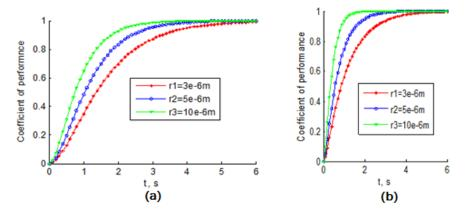
**Figure 3.** The dependence of the coefficient of performance of the active zone of corona discharge, respectively (a)- at a current density  $j = \frac{10^{-4}A}{m^2}$  and (b)- at a current density  $j = \frac{5.10^{-4}A}{m^2}$
