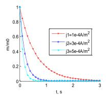
**Figure 1.** Changes in amount of charged particles as a function of the active zone corona for different values of ion current density
