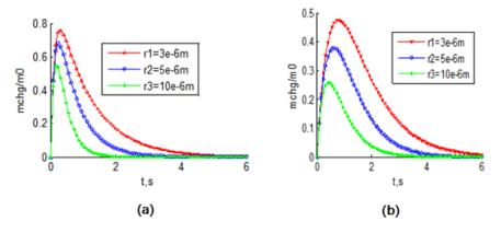
Figure 2. The amount of charged particles located in the studied space, respectively. (a)- at a current density  $j = 10^{-4} A/m^2$  and (b)at a current density  $j = 5.10^{-4} A/m^2$
