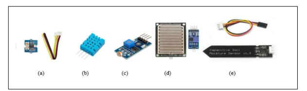
Figure 2. Grove-uv sensor (a), temperature and humidity sensor (b), ldr sensor (c), rain sensor (d), soil moisture sensor (e)
