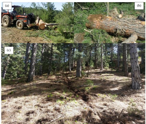
**Figure 2.** Turkish red pine timber extraction by using farm tractor: uphill winching (a), crumbs of soil left on the log (b) and damage to the soil by skidding whole tree (c)
