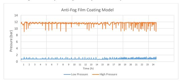
Figure 4. Time-dependent high and low pressure values of the anti-fog film coating model
