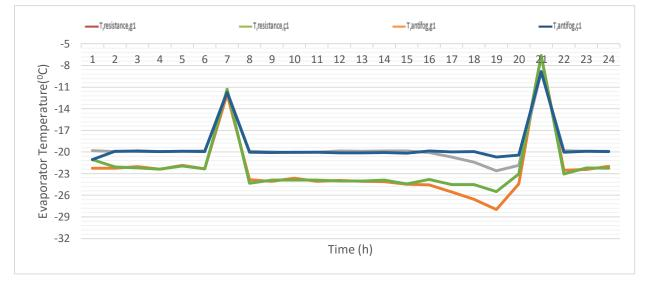
Figure 7. Variation of evaporator inlet and outlet air temperature over time
