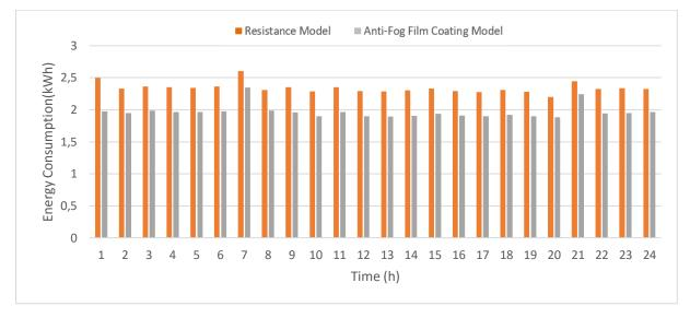
Figure 5. Energy consumption of the refrigeration system
