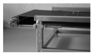
Figure 2. Shafts of carrier band
