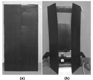
Figure 1. The box used for light insulation: (a) Closed view, (b) Open view
