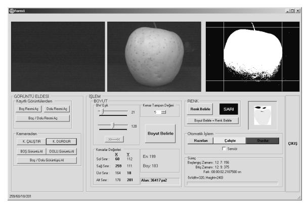
Figure 4. Inspecting yellow apple with software
