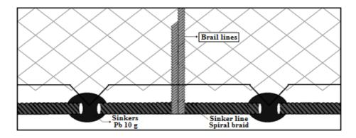
Fig 3. Sinker line and connecting to brail lines
