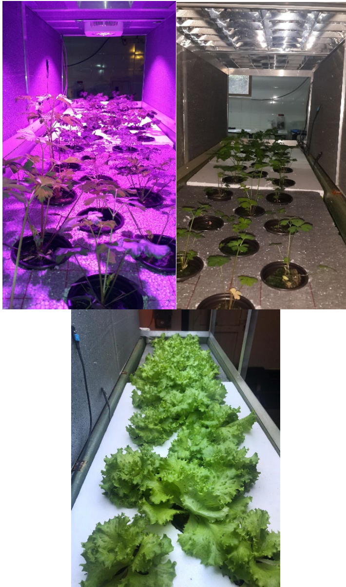
Figure 2. The plant grow beds under LED (upper left), HPS (bottom middle), and FLO (upper right) lights in the experimental aquaponics system
