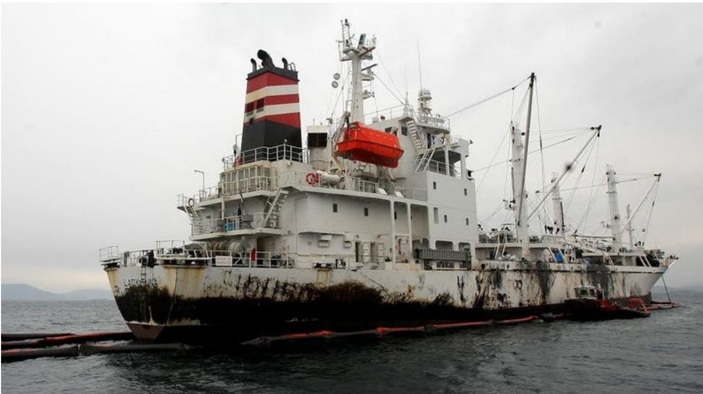
Picture 2. Booms used to control the pollution arising from M/V Lady Tuna (Anonymus, 2017c)
