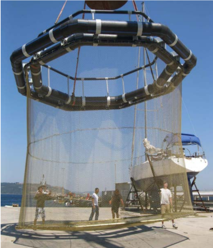
Figure 16. The completed fish cage with copper-alloy mesh being raised for inspection.
