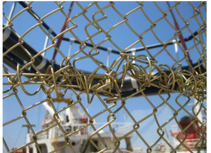
Figure 15. Seams between the side panels required additional wire support.
