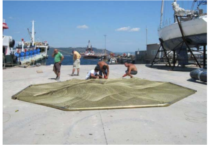
Figure 9. The side panels were folded to the inside of the cage to allow adjacent panels to be secured together.
