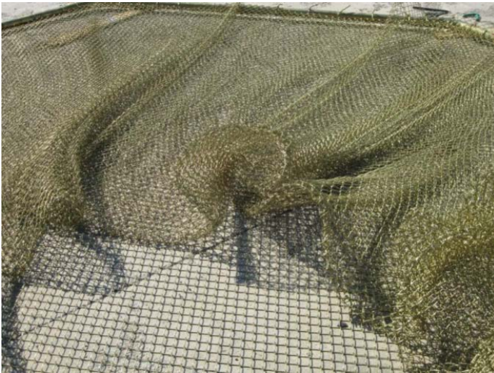
Figure 12. Side panels were folded to align the top edge of the net for attachment of the top rim
