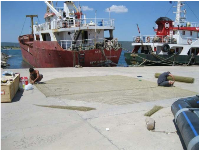
Figure 4. The corners of the bottom net panel were removed to form an octagon
