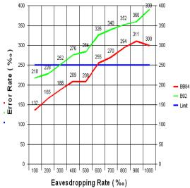
Fig. 6.2 Relationship between error rate and increasing eavesdropping rate
