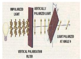
Fig.2.3 Unpolarized photons pass through first filter and gain a polarisation angle of 0 degree. This measurement randomizes these photons's pass through second fitler[1]
