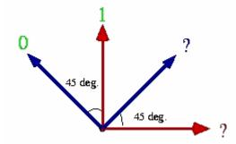
Fig. 3.3 Qubit – Polarisation matching for B92 protocol's receiving side
