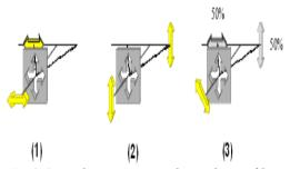
Fig. 2.4 Reading process with rectilinear filter and photons with polarisation angles of 0, 90 and 135 degrees
