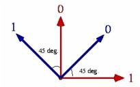
Fig. 3.1 Qubit – Polarisation matching of BB84 protocol for sending / receiving process
