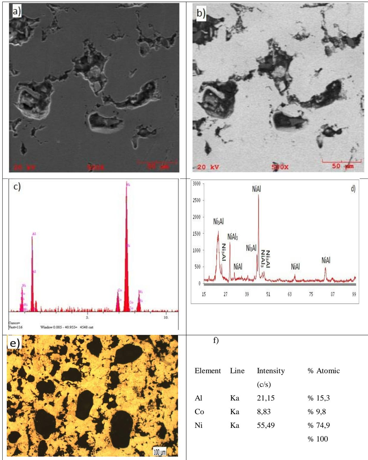
Figure 5: a) SEM, b) BSE, c) EDS graph, d) XRD, e) optical microscope image, f) EDS composition ratios of the Co reinforced NiAl alloys
