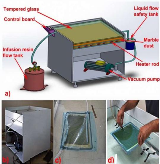
Figure 1. a) Vacuum infusion bench schematic view
