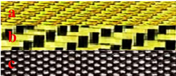
Figure 2. Fibers used in production a)Kevlar b)Aramid c)Carbon
