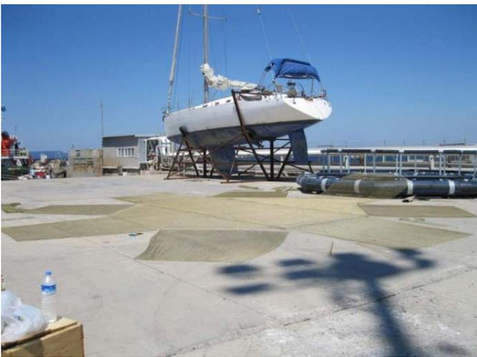
**Figure 5.** The side panels were laid out radially from bottom panel to ease assembly.
