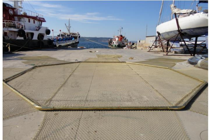
**Figure 10.** Double loop ties were placed every 20cm on the bottom net rim
