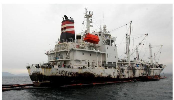
**Picture 2.** Booms used to control the pollution arising from M/V Lady Tuna (Anonymus, 2017c)
