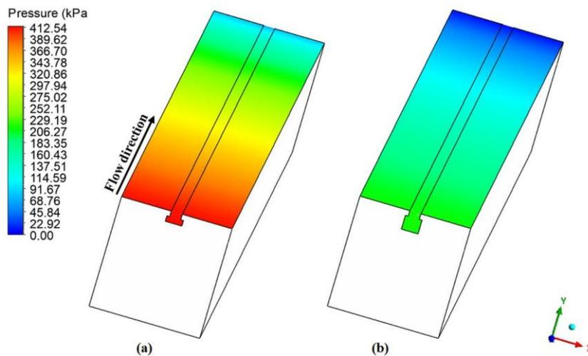
Figure 7. Contours of pressure at the cathode flow channel inlet and flow channel/GDL interface for channel configurations having a half square section with rectangular sections of (a) 0.3 x 0.1 mm and (b) 0.3 x 0.25 mm.
