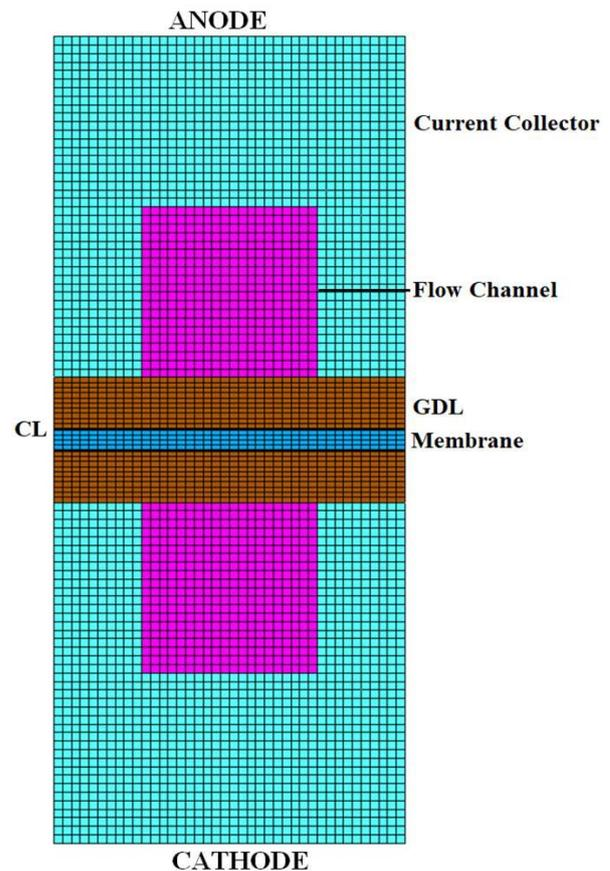
Figure 1. Grid structure and parts of PEMFC model.
