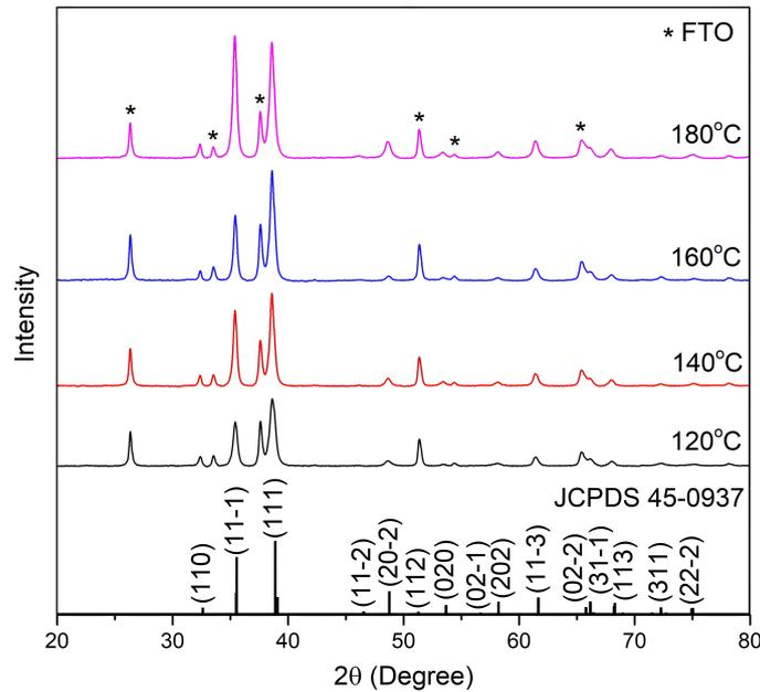
**Figure 1.** XRD patterns of CuO thin films deposited at different hydrothermal reaction temperatures
