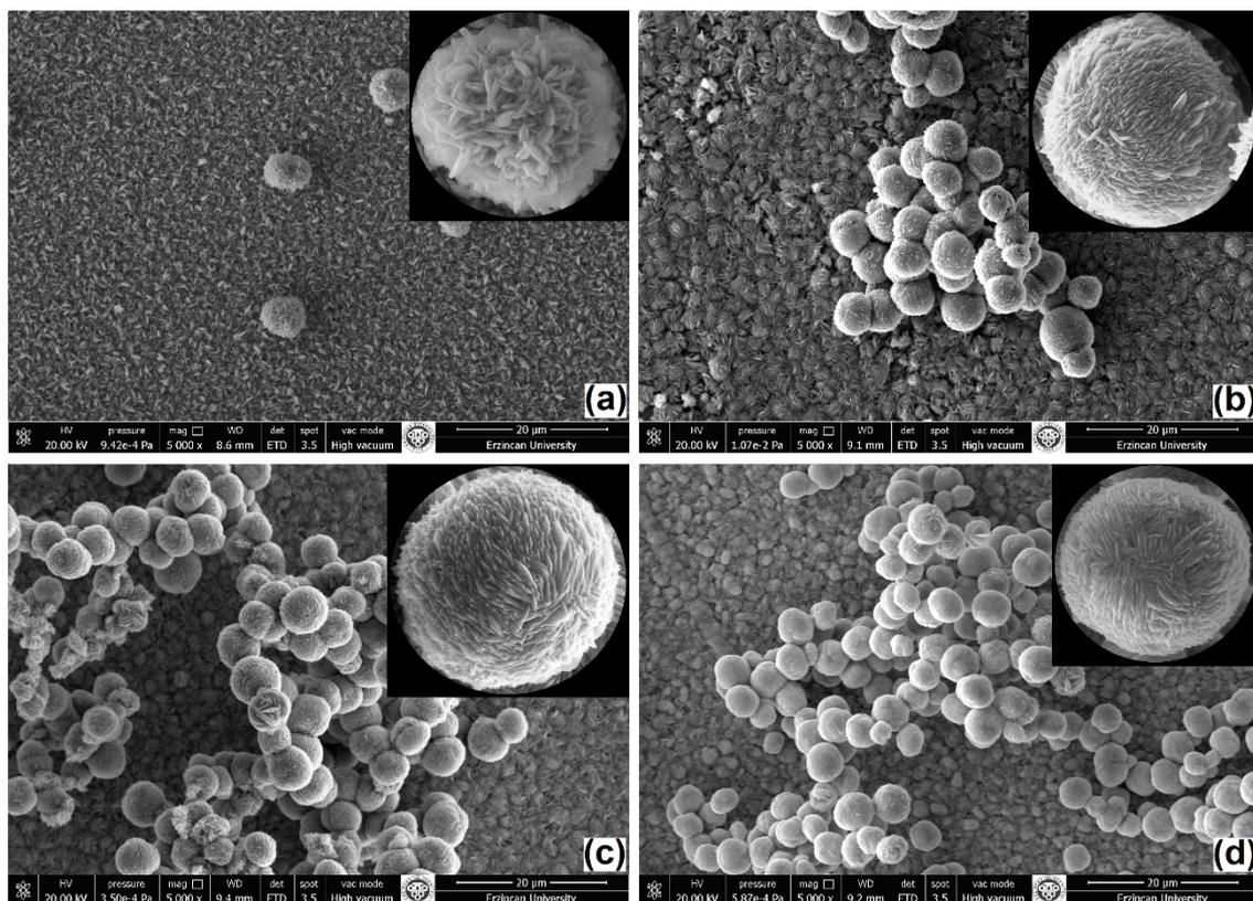
**Figure 2.** SEM images of CuO thin films deposited at different hydrothermal reaction temperatures, (a) 120°C, (b) 140°C, (c) 160°C, (d) 180°C.
