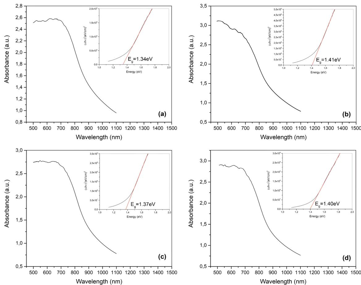
**Figure 5.** Optical absorption spectra with the variations of  $(\alpha h\nu)^2$  as a function of photon energy for CuO thin films deposited at different hydrothermal reaction temperatures, (a) 120°C, (b) 140°C, (c) 160°C, (d) 180°C.
