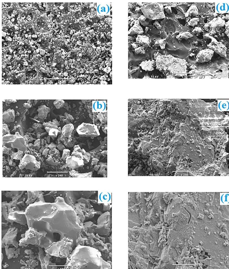
**Figure 11.** SEM images of Al(OH)<sub>3</sub> and Al<sub>2</sub>O<sub>3</sub> at different magnifications; a) Al(OH)<sub>3</sub> at 50X magnification, b) Al(OH)<sub>3</sub> at 240X magnification, c) Al(OH)<sub>3</sub> at 500X magnification, d) Al<sub>2</sub>O<sub>3</sub> at 50X magnification, e) Al<sub>2</sub>O<sub>3</sub> at 240X magnification, f) Al<sub>2</sub>O<sub>3</sub> at 500X magnification
