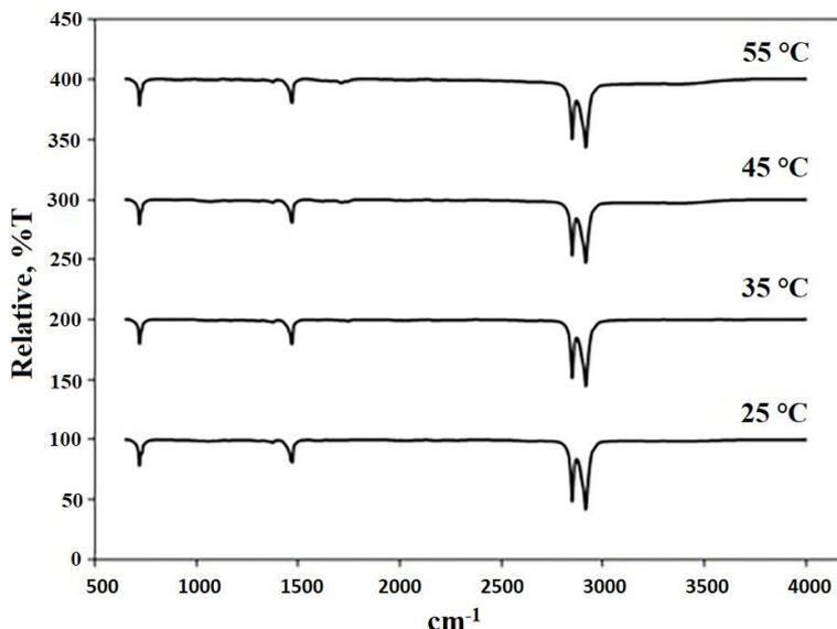
**Figure 6.** FTIR patterns of filter cakes obtained from experimental studies carried out with 6.038 M HCl and increasing temperatures
