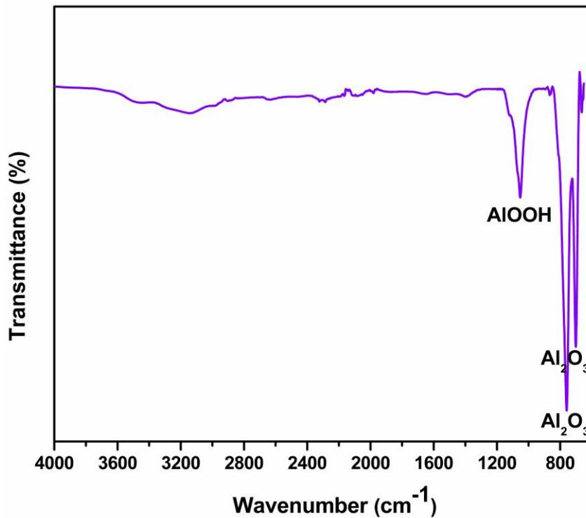
**Figure 8.** FTIR pattern of calcined Al<sub>2</sub>O<sub>3</sub>
