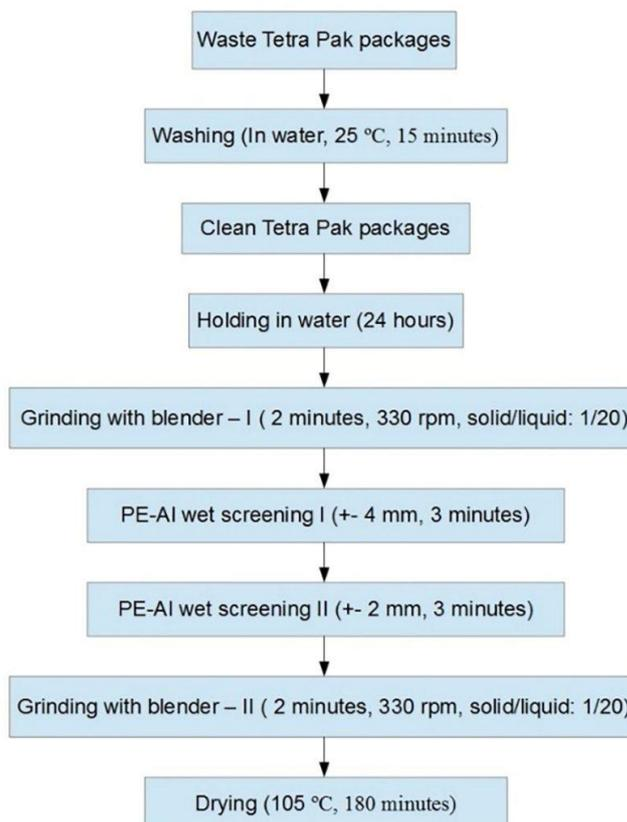
**Figure 1.** Hydropulping process flow chart
