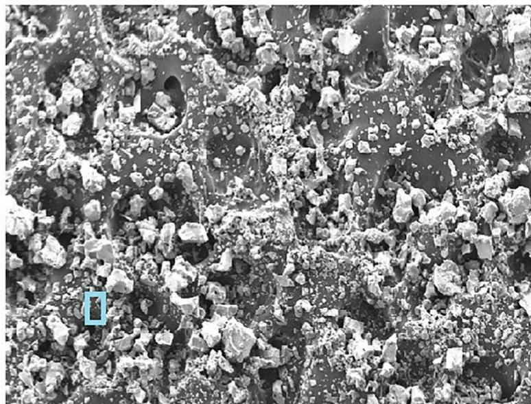
**Figure 9.** SEM image of Al(OH)<sub>3</sub>
