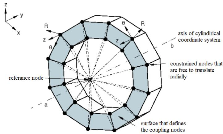
**Figure 4.** An example of coupling constraint (Abaqus documentation, 2023)
