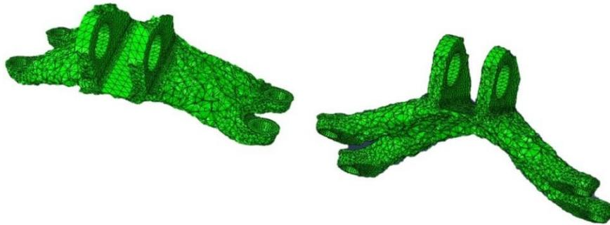
**Figure 9.** Topologically optimized shape, after 25 design cycles
