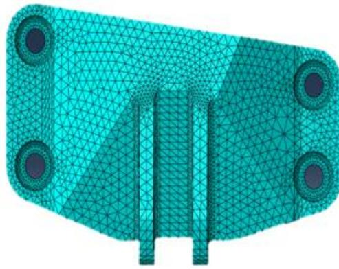
**Figure 6.** Finite element mesh structure
