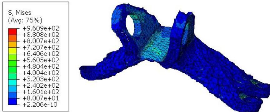
**Figure 12.** Optimized structure under Load Condition-3
