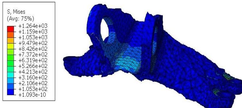
**Figure 11.** Optimized structure under Load Condition-2
