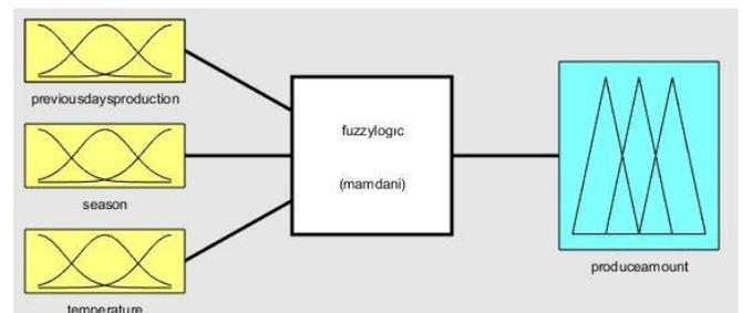
Figure 2. Fuzzy logic model of electricity production quantity
