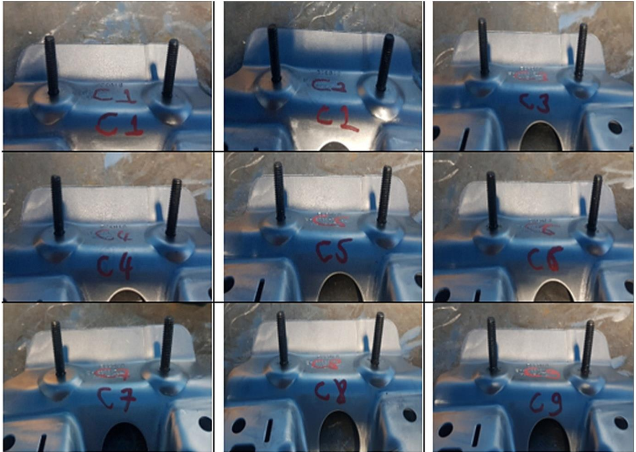
Figure 2. Test specimens made of WSS-M1A365-A11 steel with triple projection bolts welded for the study
