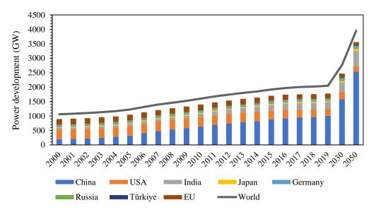
Figure 4. Power perspectives and projections of CTPPs in the world
