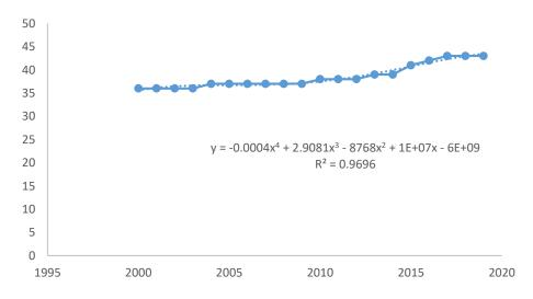
Figure 19. Power Capacity Progress and Projections of CTPPs for Russia
