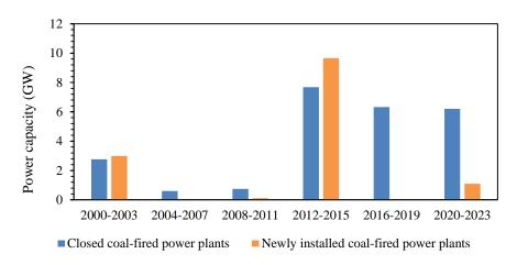
Figure 16. Nominal power values of CTPPs closed and newly established in Germany
