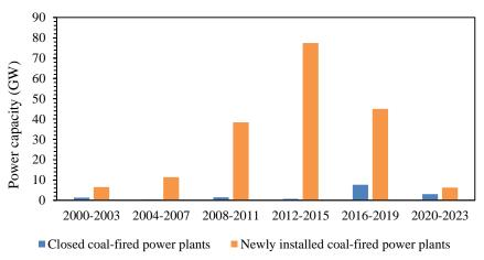
Figure 9. Nominal power values of CTPPs closed and newly installed in India
