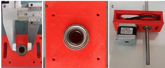
**Figure 8.** Sample application manufacturing a) rolling bearing on the successfully machined workpiece b) bearing sample view c.) manufacturing completed model.
