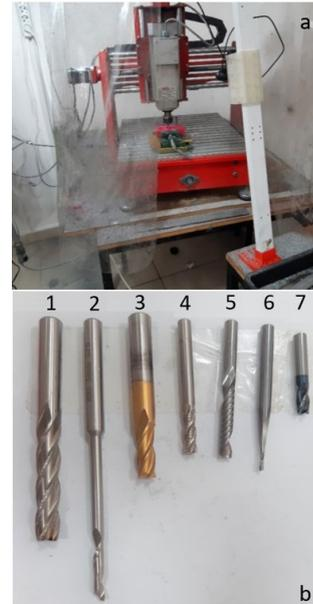
**Figure 4.** a) Desktop CNC milling machine b) end milling cutters used in processing.
