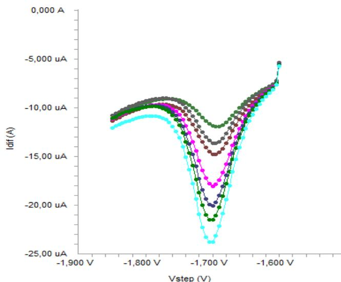
**Figure 3.** SWV voltammograms for different concentration of MX (10, 20, 40, 60, 70, 80 and 90  $\mu\text{g}/\text{mL}$ ) in SEs ( $\text{CH}_3\text{COOH}/\text{CH}_3\text{COONa}$  buffer (0.2 M, pH 4.85)/NaOH (0.2 M) (v:v, 1:1).
