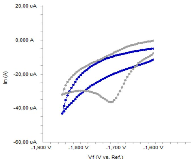
**Figure 2.** CVs of GCE in SEs (CH<sub>3</sub>COOH\CH<sub>3</sub>COONa buffer (0.2 M, pH 4.85)/NaOH (0.2 M) (v:v, 1:1) containing 50 µg/mL MX
