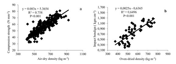
Figure 2. Relationships between (a) density and compression strength and (b) and impact bending
