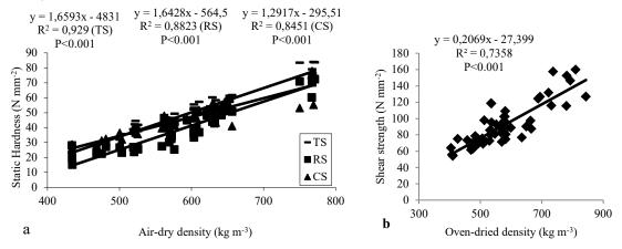
Figure 3. Relationship between (a) density and hardness, (b) density and shear strength
