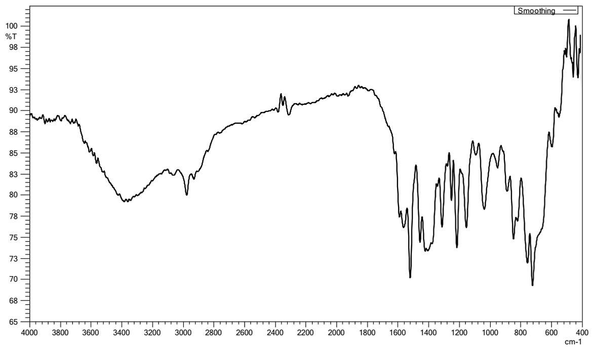
**Figure 5.** FT-IR spectrum of the L-Co complex
