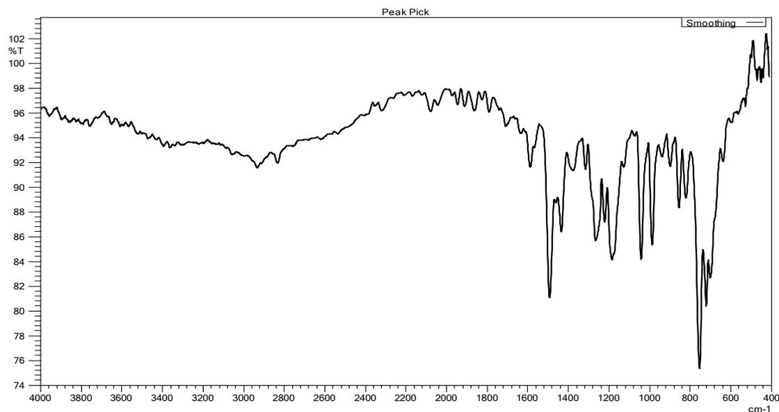
**Figure 2.** FT-IR spectrum of the ligand (H<sub>2</sub>L)
