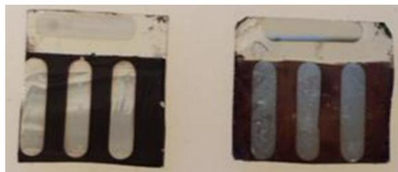
**Figure 2.** Illustration of the PSC of  $\text{ITO}/\text{TiO}_2/\text{CH}_3\text{NH}_3\text{PbI}_3/\text{P3HT}/\text{Ag}$ , and (b) the Reel images of  $\text{ITO}/\text{AA}-\text{TiO}_2/\text{CH}_3\text{NH}_3\text{PbI}_3/\text{P3HT}/\text{Ag}$ (left) and  $\text{ITO}/\text{AA}-\text{TiO}_2/\text{m}-\text{TiO}_2/\text{CH}_3\text{NH}_3\text{PbI}_3/\text{P3HT}/\text{Ag}$ (right)
