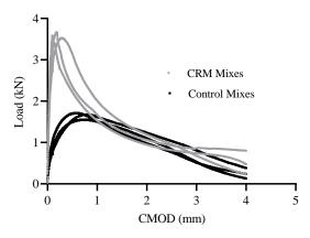
Figure 7. The work of fracture plots
