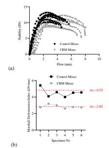
Figure 6. Marshall deformation index in specimens
