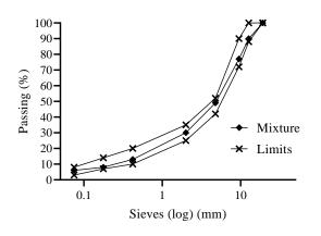
Figure 1. Gradation limits for HMA
