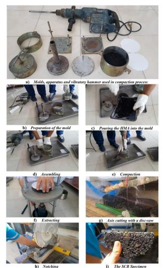
**Figure 3.** Preparation steps of the SCB specimen
