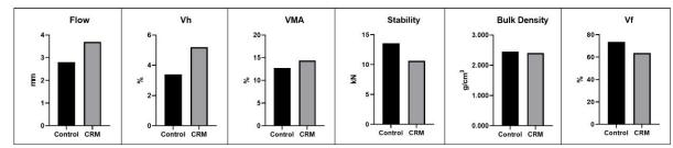
Figure 5. Marshall test results
