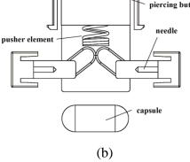
Figure 2. Modified one-button dry powder inhaler, (a) general view, (b) components of device
