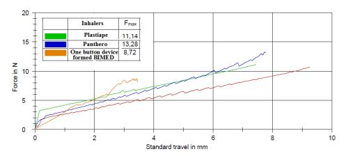
Figure 4. Force and needle travel required to puncture the capsule
