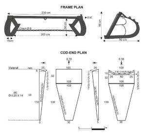
Figure 3. Technical plan of beam trawl cod-end
