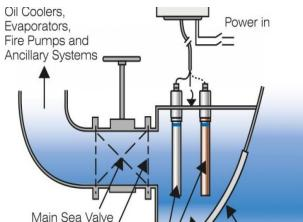
Fig. 7. Seawater cooler working principle (Vyasmetal, 2022).
