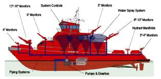
Fig. 10.Fire suppression system ship fire extinguishers (URL 5).
