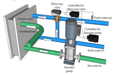
Fig. 4 Configuration of the ship's central cooling system (Lee et al., 2021).
