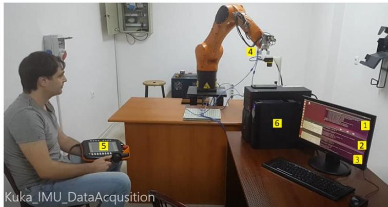
Figure 6 Experimental setup for simultaneous recording of Kuka and IMU data.
