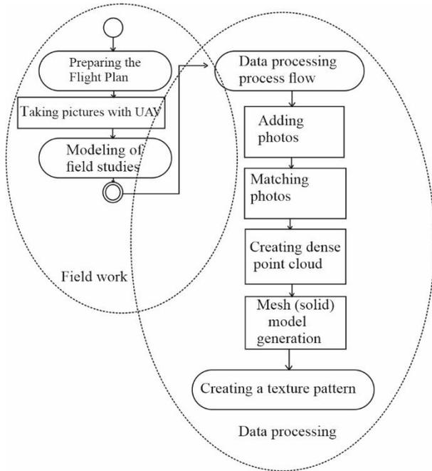
**Figure 6.** Processes in the UAV photogrammetry method
