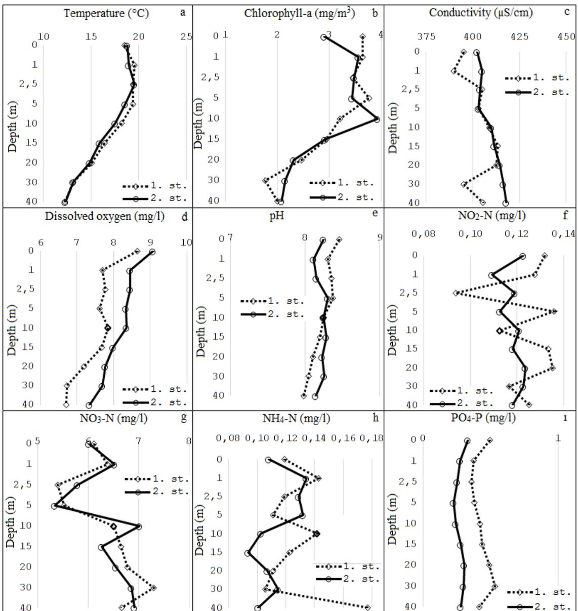
**Figure 4:** Water quality parameters in different depth in cage and reference stations in Kozan Dam Lake
